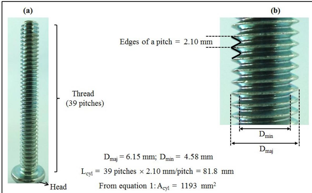
FIGURE 1: (a) Photograph showing different parts of a machine screw: head and thread, and (b) enlarged part of the same photograph showing shape and size of the pitches.
