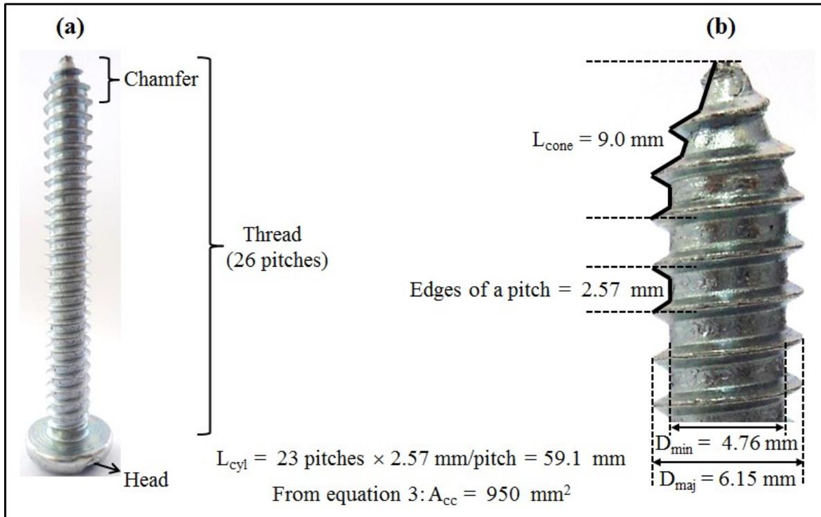
FIGURE 2: (a) Photograph showing different parts of a sheet metal screw, and (b) enlarged part of the same photograph showing shape and size of the pitches (6.15 mm: 305 pixels).
