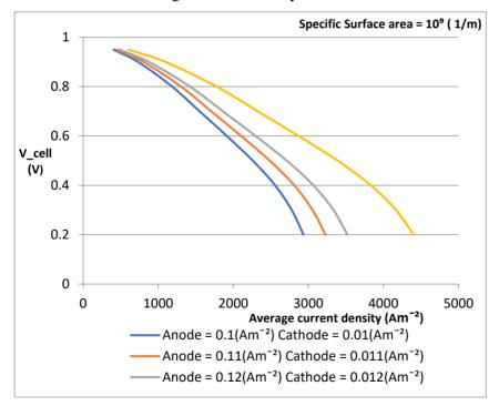
Then the same variation is also studied by changing the specific surface area of the anode and the cathode to  $10^9 m^{-1}$  (keeping operating temperature of SOFC at 800°C). The variations showed a similar trend but the magnitudes of the power output and the cell voltage changed (decreased) quite significantly. The power characteristics for the various values of exchange current density were obtained as follows.
