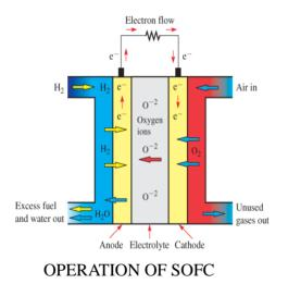
Hence, in a fuel cell the energy released in chemical reaction is directly converted to the electrical energy.
