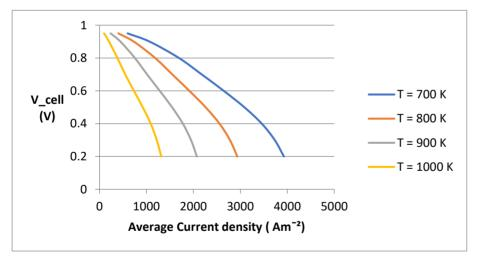
As is evident from the graph, the cell voltage decreases as the temperature of the SOFC is increased
