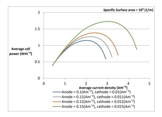
From the graph it can be seen that as the specific surface area decreases, the average current density and the average cell power decrease. However increase in the exchange current density increases the average output power of the cell.
