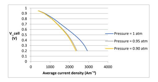
The results obtained are quite show a similar trend that the variation of pressure from 1 atmosphere to 0.95 atmosphere changed the polarization curve significantly, but further reduction
