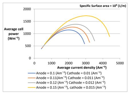
From the graphs, it is clear that as the exchange current density increases, the output power of the SOFC also increases. Even a slight change in the exchange current density brings a significant change in the output power.
