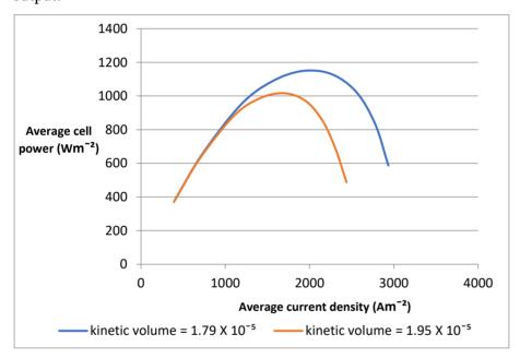
Similarly, the polarization curve was also plotted for the variation in the kinetic volume of the inert gas at 800°C. The polarization characteristics also show that the output cell voltage decreases as the kinetic volume of inert gas increases.
