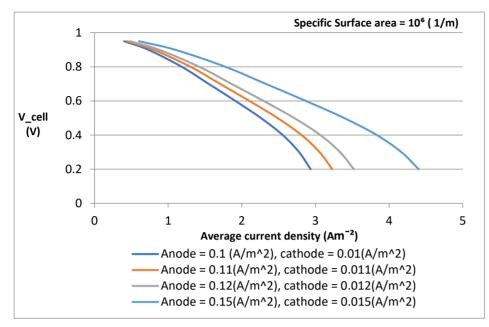
It is clear from the above, that as the specific surface area decreases, the average current density output of the cell for given cell voltage decreases drastically. However, increase in exchange current density of the anode and the cathode increase the cell voltage for a given exchange current density.
