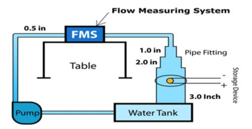
FIGURE 3. Geometrical Layout of Working Model with Closed Channel-Based Energy Harvesting System
