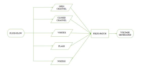
FIGURE 1. Block Diagram of Fluidic Energy Harvesting with Different Experimental Set-ups
