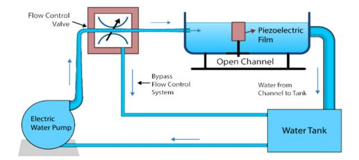
FIGURE 2. Geometrical Layout of Working Model with Open Channel- Based Energy Harvesting System
