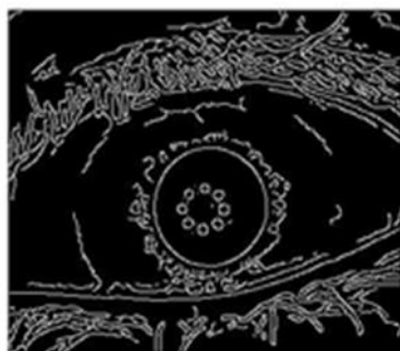
Fig 2. The result of canny edge detection.
