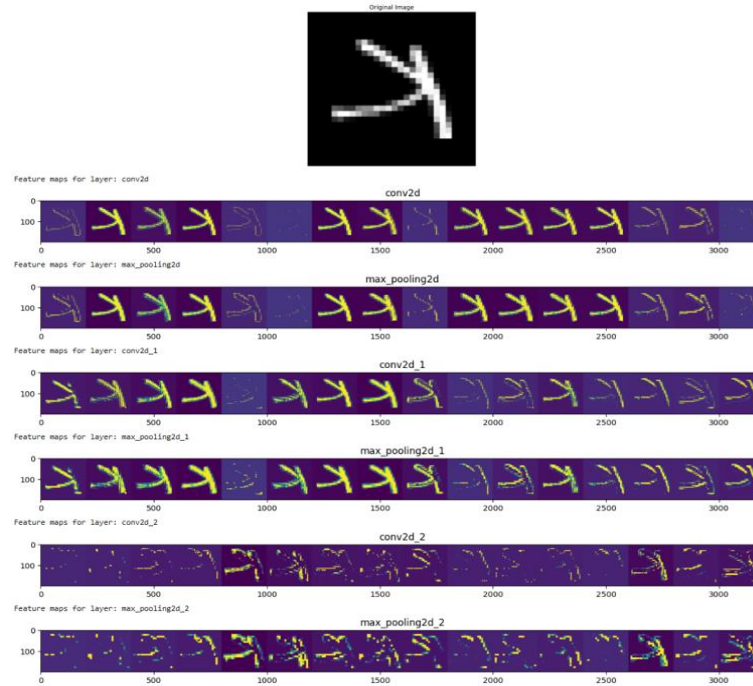
FIGURE 11. Feature map visualization of CNN layers in the Custom LiteBinaryNet architecture for the letter “K”
