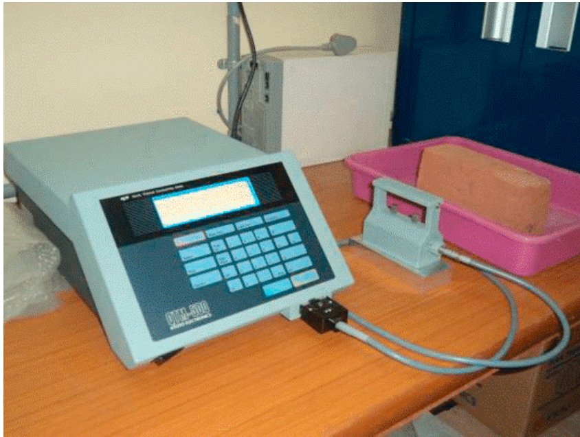
FIGURE 3. The image showing a device to measure thermal conductivity
