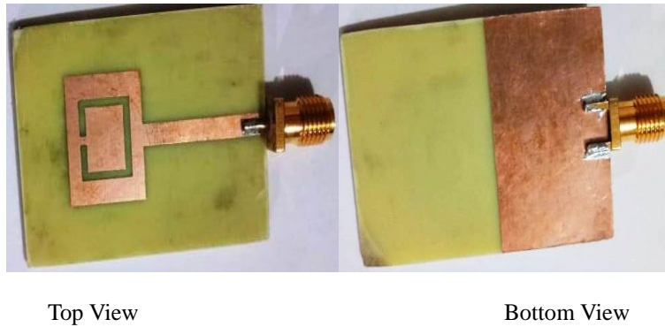
FIGURE 5. Schematic diagrams of the fabricated proposed antenna.
